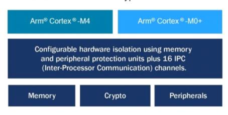
Pictured is a block diagram showing the integrated security in Cypress' PSoC 6 microcontrollers, which delivers the highest level of protection as defined by Arm's Platform Security Architecture. (Graphic: Business Wire)
